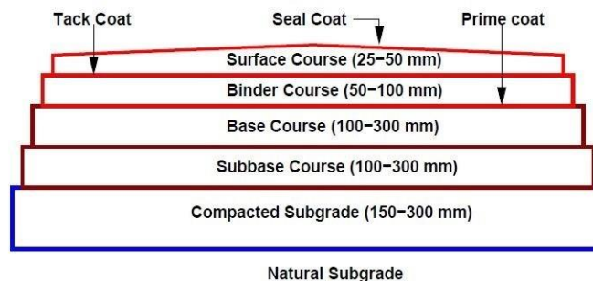
Typical cross section of a flexible pavement
