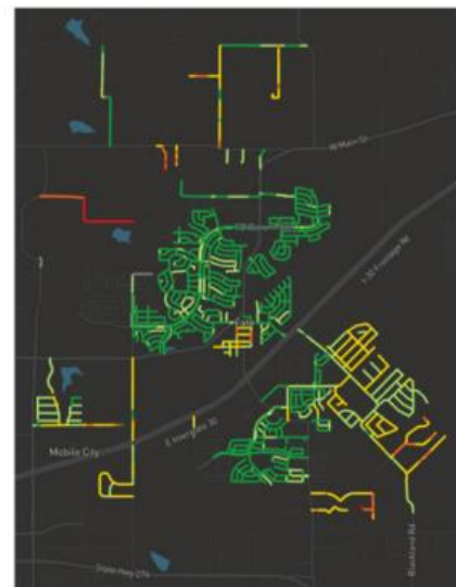
Figure 2. Pavement Condition Assessment Map The map uses a color-coded system to indicate Fate road conditions. Green: Roads in good condition with minimal wear. Yellow: Roads showing moderate deterioration, likely requiring maintenance soon. Orange/Red: Roads in poor condition, with significant wear, cracks, or structural failures, likely requiring major repairs or full reconstruction.
